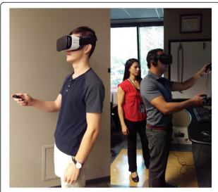
**Fig. 1** Samsung Oculus Gear VR with supplemental hand controller (left) and Oculus Rift (right)
