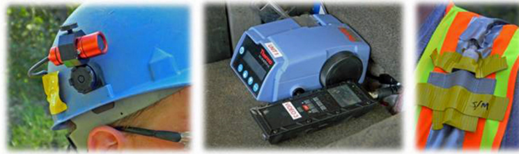
Fig. 1 (From left to right) video camera attached to helmet, dust monitor and video monitor, and safety vest to hold instrumentation
