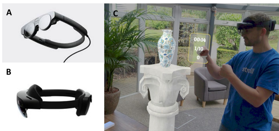
Fig. 1 Augmented-reality (AR) glasses (Magic Leap 2 (A) and HoloLens 2 (B)) for performing gait-and-balance exercises at home using Reality DTx ® therapeutic exergames. In (C), 'Smash' is illustrated, an AR boxing game promoting weight shifts, dynamic balance, turning, and walking with direct feedback on task duration, number of required punches, and number of smashed holograms like the depicted vase)
